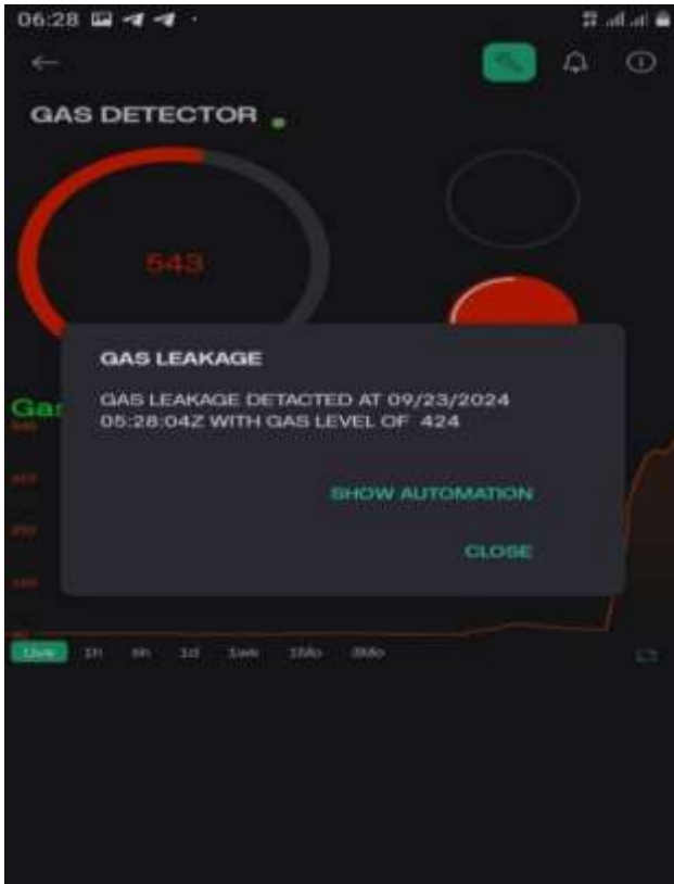
Figure 6: High Gas Concentration
